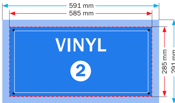
VINYL Corner / Detail: position for drilling and clips
